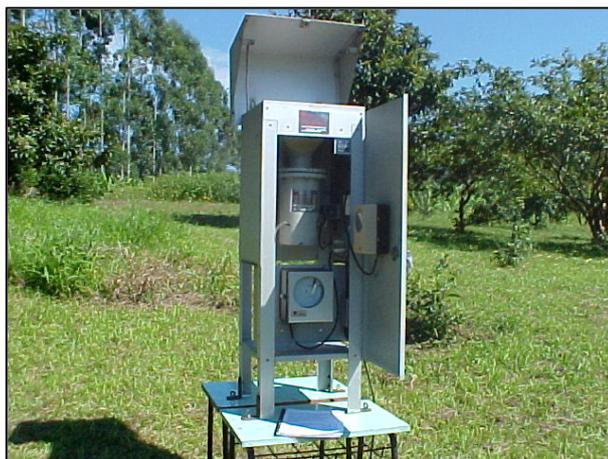
Figura 6-10 - Amostrador AGV PTS (ENERGÉTICA).
